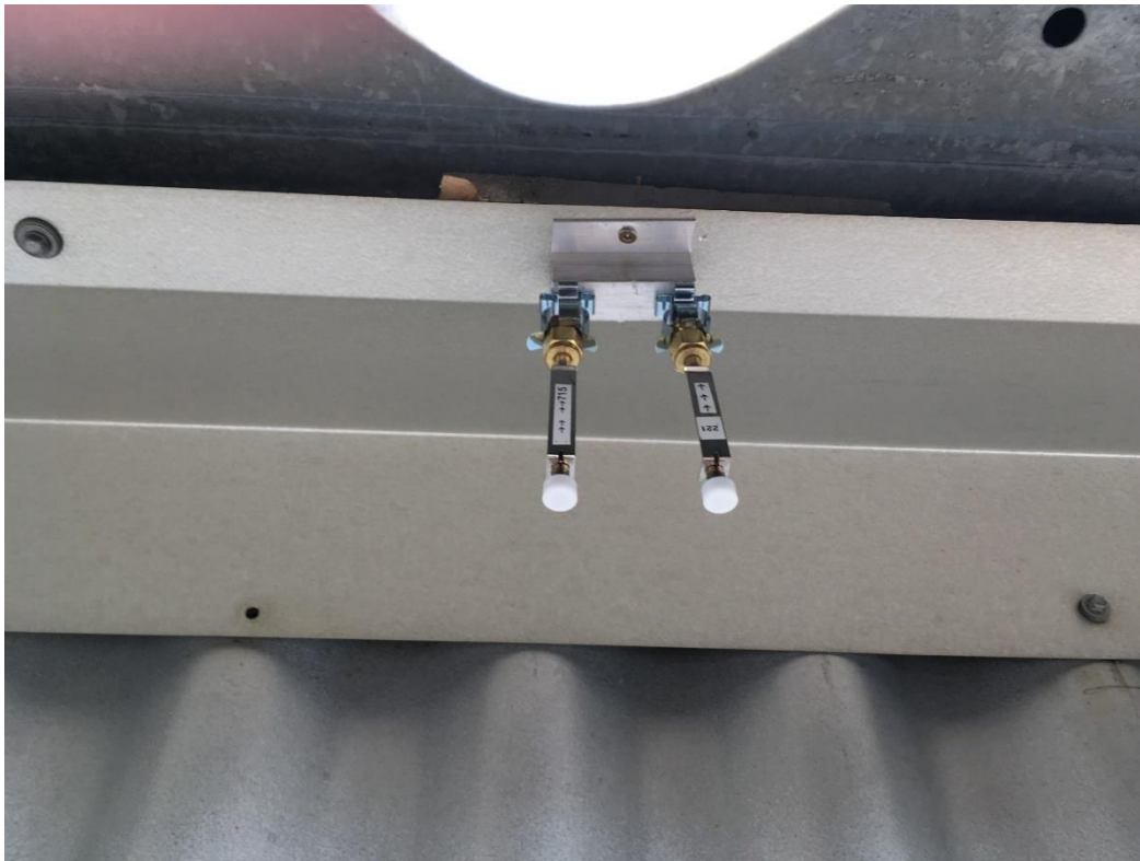
Figure 5 Tenax tubes at site USI-1, outside baghouse.
